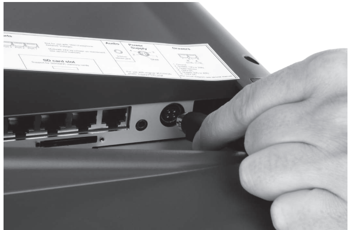
Fig. 11: Putting the power cable plug to the power connection
