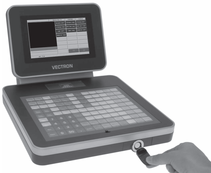
Fig. 19: Approaching the key to the operator lock
